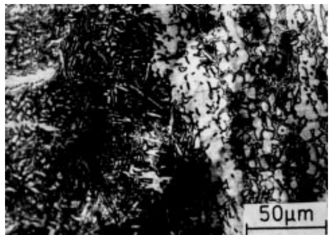
Fig. 4 Gas tungsten arc weldment and heat affected zone (pure argon and 5% N 2 )
